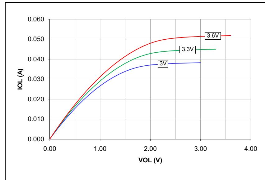
**FIGURE 32-8: VOL – 16x DRIVER PINS**
