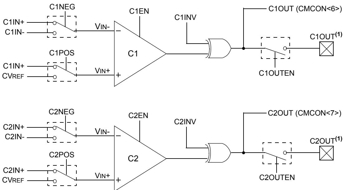
**Note 1:** This peripheral's outputs must be assigned to an available RPn pin before use. Refer to **Section 11.6 "Peripheral Pin Select"** for more information.
