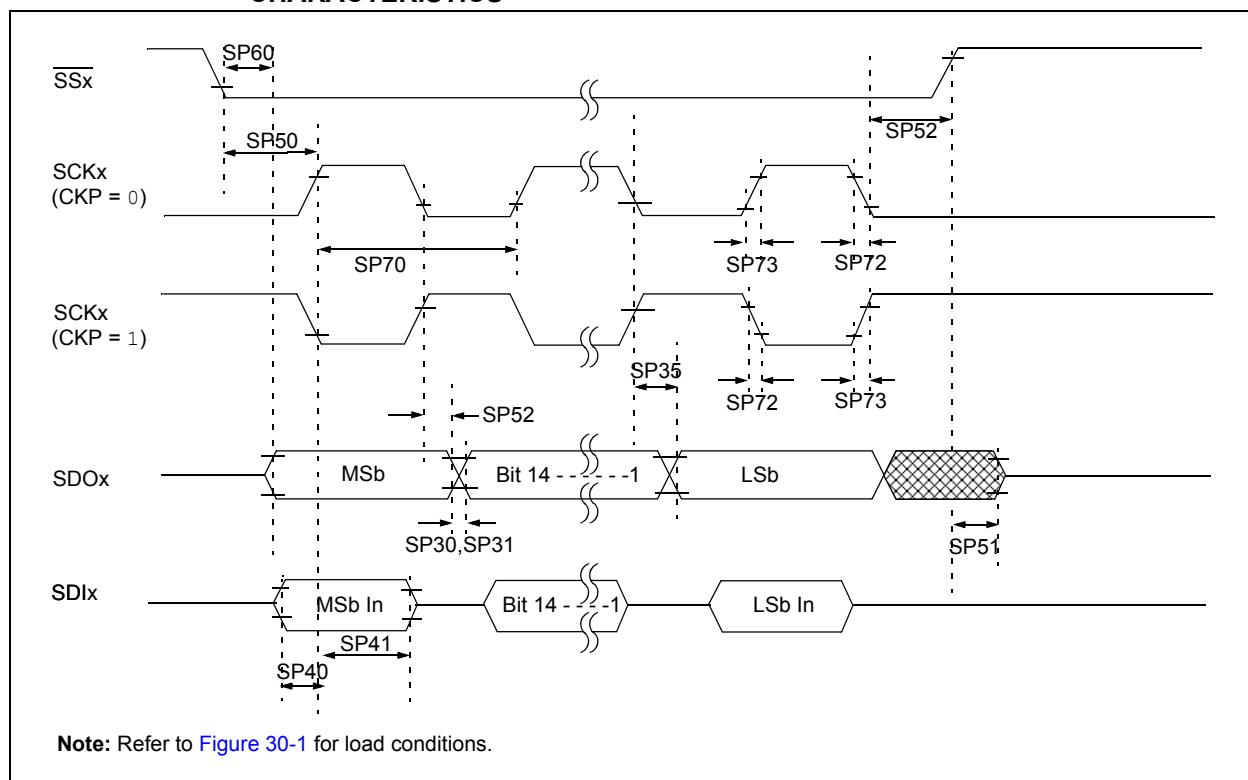
**TABLE 30-33: SPI<sub>x</sub> SLAVE MODE (FULL-DUPLEX, CKE = 1, CKP = 1, SMP = 0) TIMING REQUIREMENTS**
