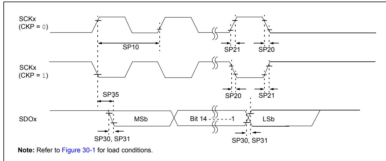
FIGURE 30-10: SPI<sub>x</sub> MASTER MODE (HALF-DUPLEX, TRANSMIT ONLY CKE = 1) TIMING CHARACTERISTICS
