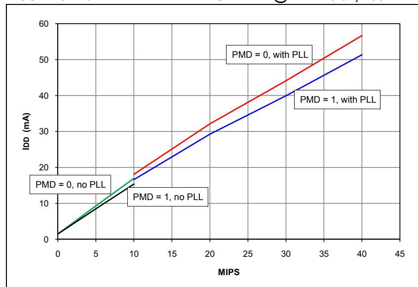
**FIGURE 32-12: TYPICAL IIDLE CURRENT @ VDD = 3.3V, +85°C**
