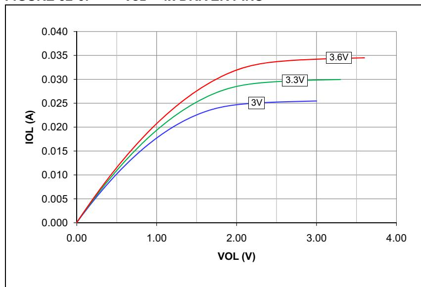
**FIGURE 32-7: VOL – 8x DRIVER PINS**
