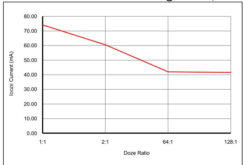
**FIGURE 32-10: TYPICAL IDD CURRENT @ VDD = 3.3V, +85°C**
