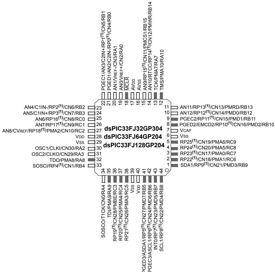
**Note 1:** The RPx pins can be used by any remappable peripheral. See [Table 1](#) in this section for the list of available peripherals.
