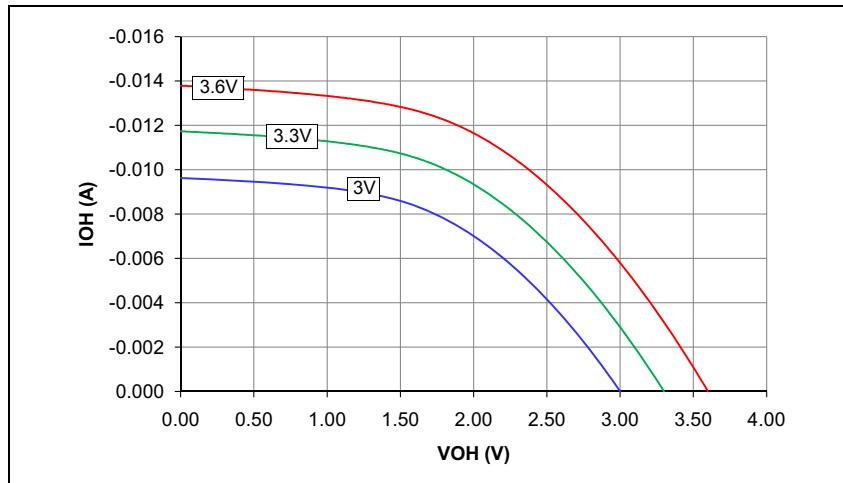
**FIGURE 32-3: V<sub>OH</sub> – 8x DRIVER PINS**
