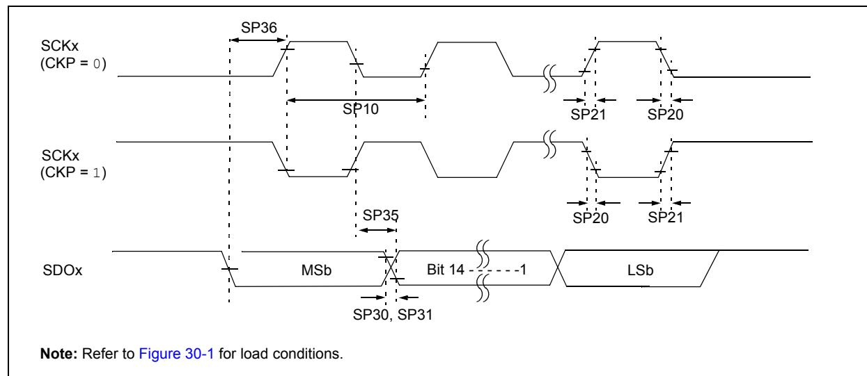
**TABLE 30-29: SPI<sub>x</sub> MASTER MODE (HALF-DUPLEX, TRANSMIT ONLY) TIMING REQUIREMENTS**
