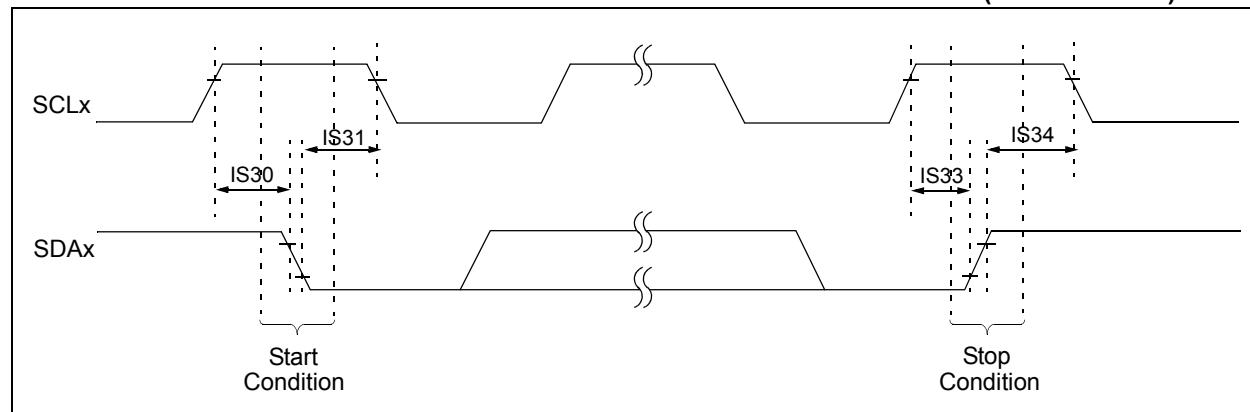
**FIGURE 30-20: I<sup>2</sup>C<sub>x</sub> BUS DATA TIMING CHARACTERISTICS (SLAVE MODE)**
