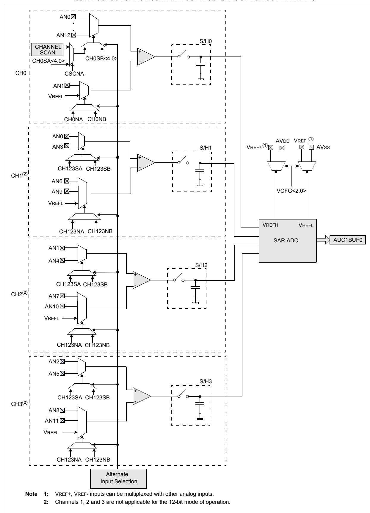
**FIGURE 21-2: ADC1 MODULE BLOCK DIAGRAM FOR dsPIC33FJ32GP302,
