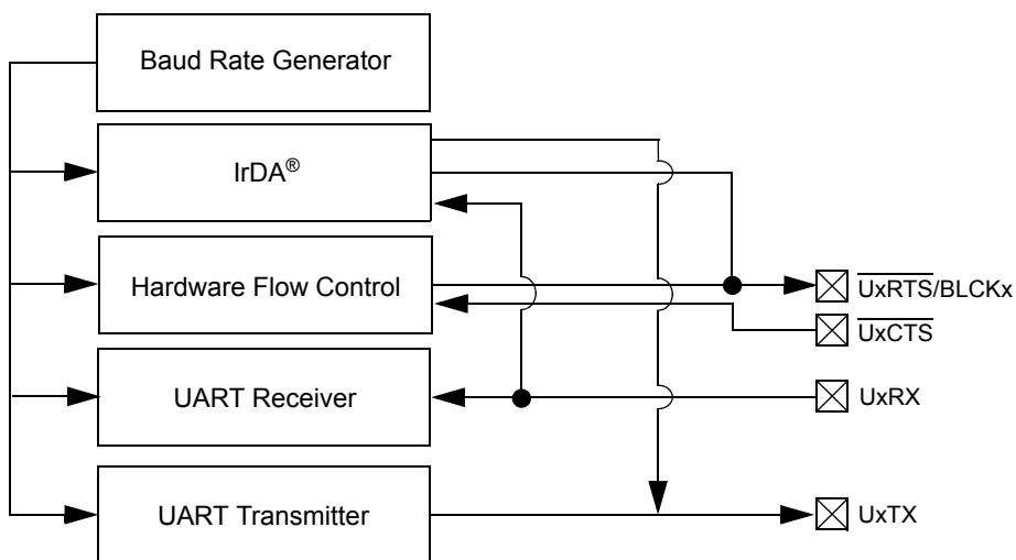
**Note 1:** Both UART1 and UART2 can trigger a DMA data transfer.
