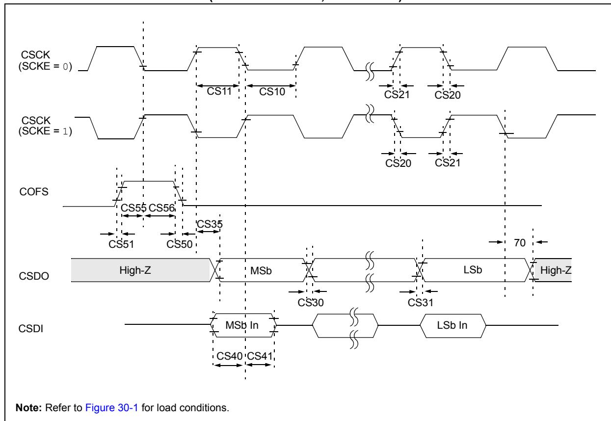
**TABLE 30-38: DCI MODULE (MULTI-CHANNEL, I<sup>2</sup>S MODES) TIMING REQUIREMENTS**
