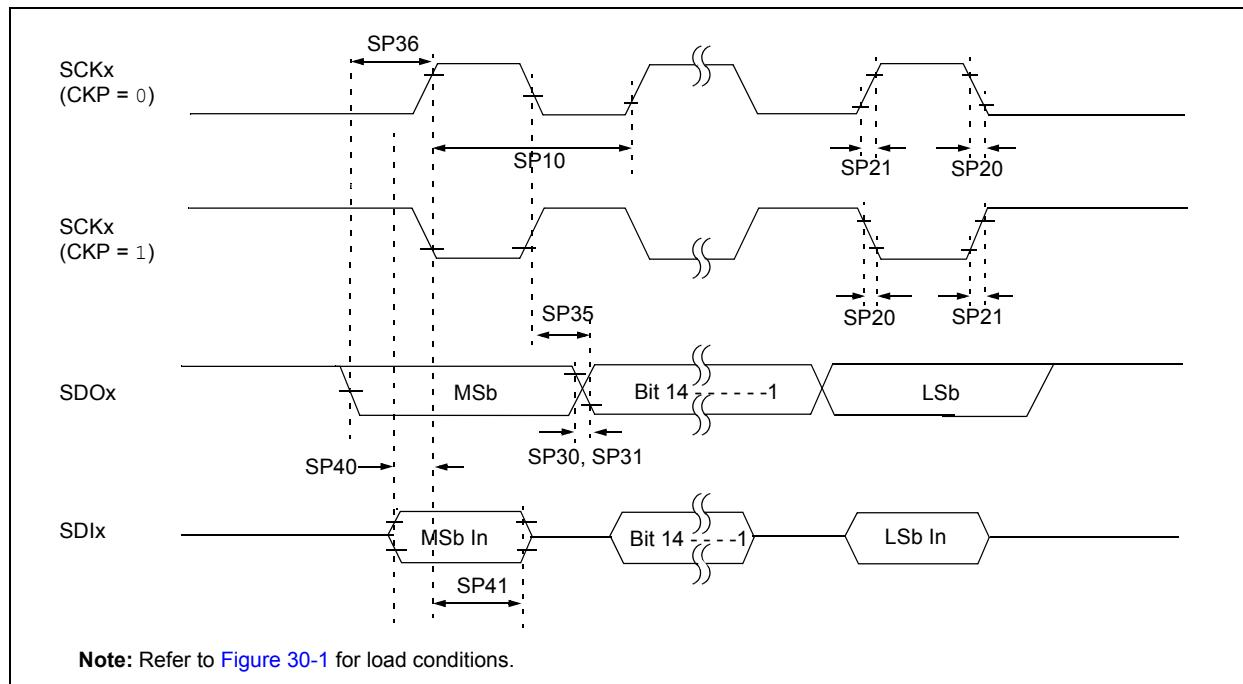
**TABLE 30-30: SPI<sub>x</sub> MASTER MODE (FULL-DUPLEX, CKE = 1, CKP = x, SMP = 1) TIMING REQUIREMENTS**
