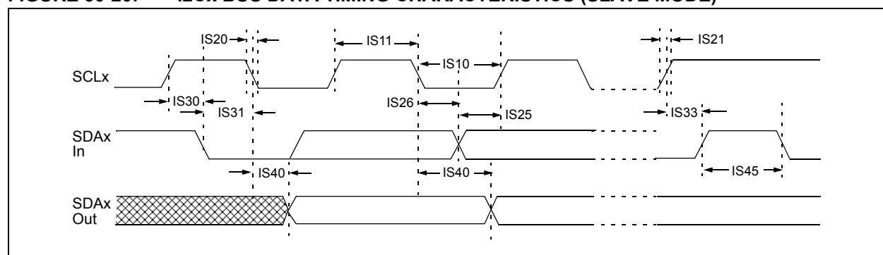
TABLE 30-37: I<sup>2</sup>Cx BUS DATA TIMING REQUIREMENTS (SLAVE MODE)
