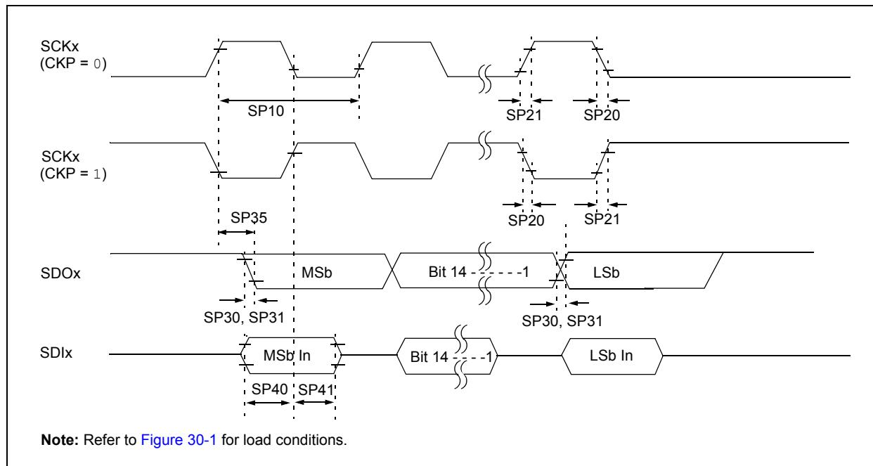
**TABLE 30-31: SPI<sub>x</sub> MASTER MODE (FULL-DUPLEX, CKE = 0, CKP = x, SMP = 1) TIMING REQUIREMENTS**
