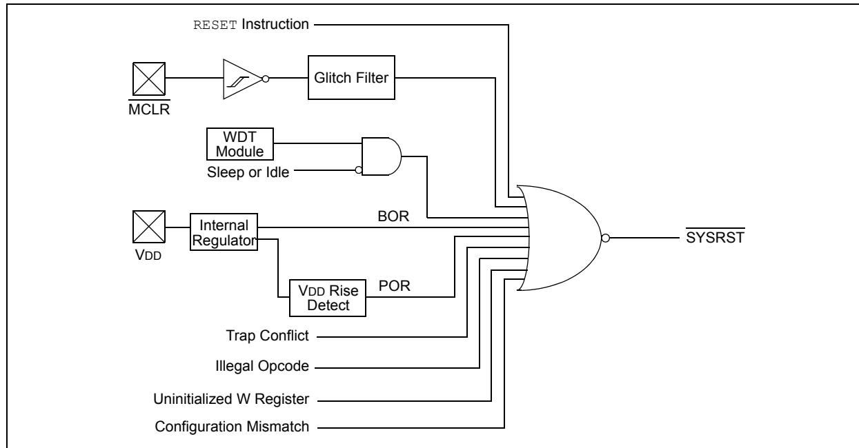
A simplified block diagram of the Reset module is shown in [Figure 6-1](#).
