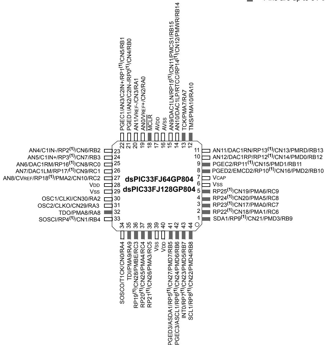
**Note 1:** The RP<sub>x</sub> pins can be used by any remappable peripheral. See [Table 1](#) in this section for the list of available peripherals.
