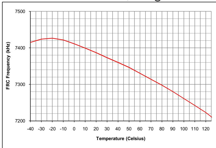
**FIGURE 32-14: TYPICAL LPRC FREQUENCY @ V<sub>DD</sub> = 3.3V**
