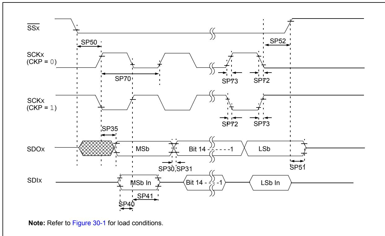
**TABLE 30-34: SPI<sub>x</sub> SLAVE MODE (FULL-DUPLEX, CKE = 0, CKP = 1, SMP = 0) TIMING REQUIREMENTS**
