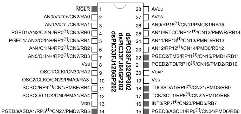
**Note 1:** The RPx pins can be used by any remappable peripheral. See [Table 1](#) in this section for the list of available peripherals.
