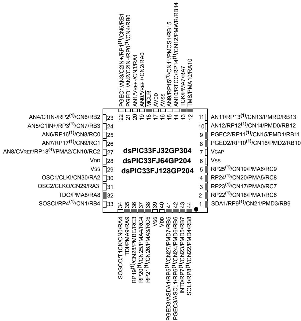
**Note 1:** The RPx pins can be used by any remappable peripheral. See [Table 1](#) in this section for the list of available peripherals.
