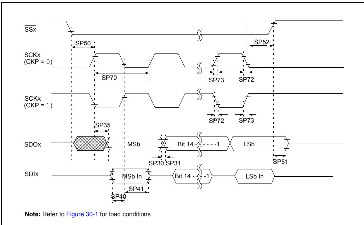
**TABLE 30-35: SPI<sub>x</sub> SLAVE MODE (FULL-DUPLEX, CKE = 0, CKP = 0, SMP = 0) TIMING REQUIREMENTS**
