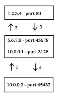
Squid should be configured so that it only listens for requests on it's internal interface, if it were listening on all interfaces I could go to 5.6.7.8 port 3128 and request http://10.0.0.2/, or any internal machine for that matter and view www content on your internal network. You want something like this in your squid.conf file:
